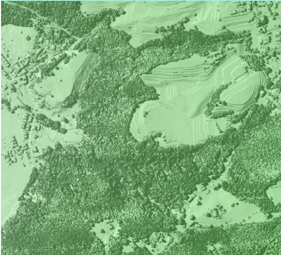
Digital Surface Model ( DSM ) derived from Laser Scanner raw data with forests and buildings
